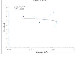
Figure 13 Strain rate influence on the stress at the strain 0.1. Penetration by the flat – ended cylinder indenter of diameter 8 mm
