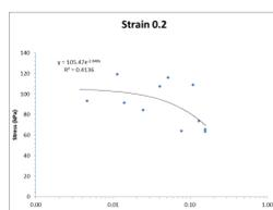
Figure 5 Strain rate influence on the stress at the strain 0.2. Compression between two parallel plates
