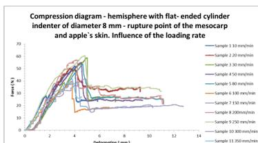
Figure 9 The influence of the loading speed on the force during penetration of the hemisphere by the flat – ended cylinder indenter of the diameter 8 mm. Rupture points of the mesocarp and the apple's skin
