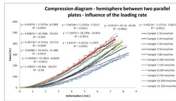
Figure 2 The influence of the loading speed on the force during the hemisphere compression between two parallel plates
