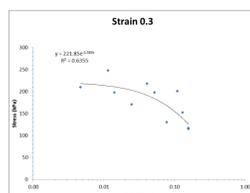
Figure 6 Strain rate influence on the stress at the strain 0.3. Compression between two parallel plates
