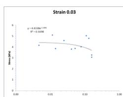
Figure 11 Strain rate influence on the stress at the strain 0.03. Penetration by the flat – ended cylinder indenter of diameter 8 mm
