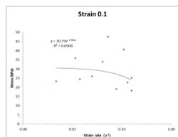
Figure 4 Strain rate influence on the stress at the strain 0.1. Compression between two parallel plates
